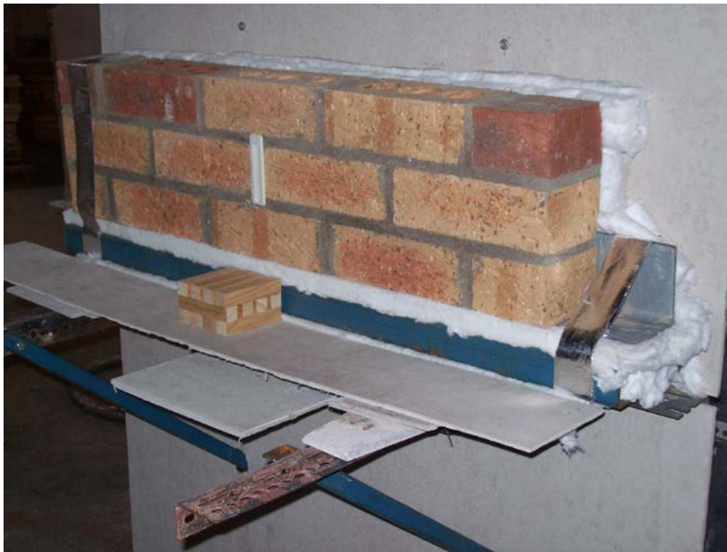
Figure 3: Weepguard as installed in wall for testing to AS 1530.8.1.
