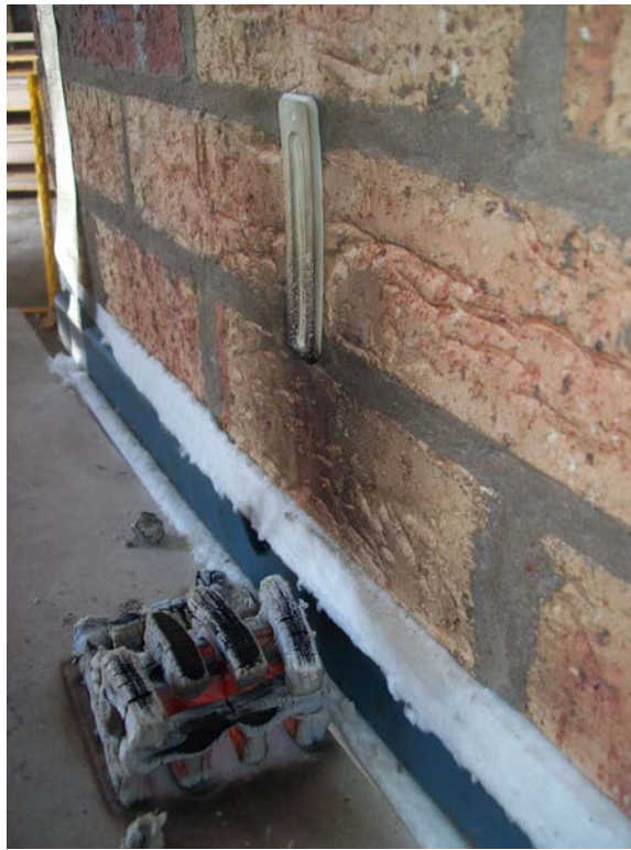
Figure 12: Weepguard/wall specimen at 20 minutes.
