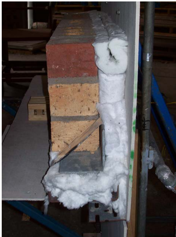
Figure 4: Side view of Weepguard/wall specimen installation showing insulation of cavity at the end and top of the sample.
